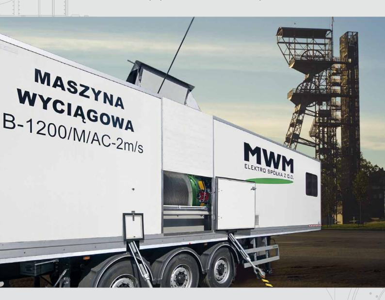
Mobile hoisting machine – driving unit of mining shaft hoist, having been additionally equipped, it may serve as complete mining shaft hoist.
